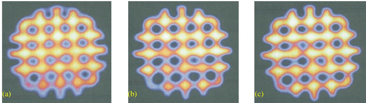
**Fig. 5 (a), (b) and (c) Show the transverse images of linearity insert (a) without, (b) with Cu 0.125 mm and (c) with Al 0.2 mm material filter, gamma camera installed with LEHR collimator.**
