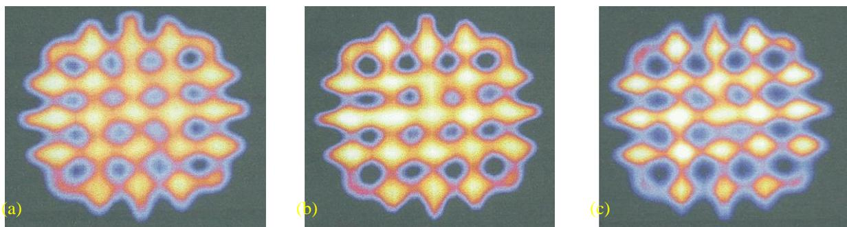
**Fig. 4 (a), (b) and (c) Show the transverse images of linearity insert (a) without, (b) with Cu 0.125 mm and (c) with Al 0.2 mm material filter, gamma camera installed with LEGP collimator.**
