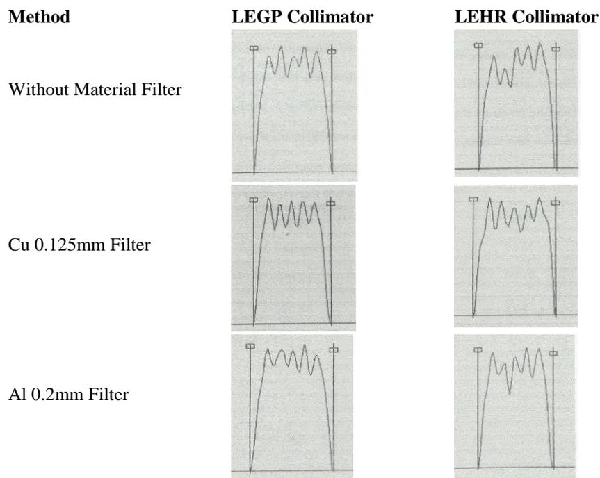
**Fig. 6 Shows the count profiles of a horizontal/vertical area in the middle of the cross grid of the linearity insert with and without material filter Cu 0.125mm and Al 0.2mm using LEGP and LEHR collimators.**
