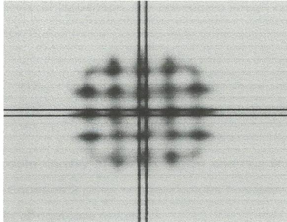
**Fig. 3 Show the selection of horizontal/vertical lines through the centre of the cross grid of the linearity insert image.**
