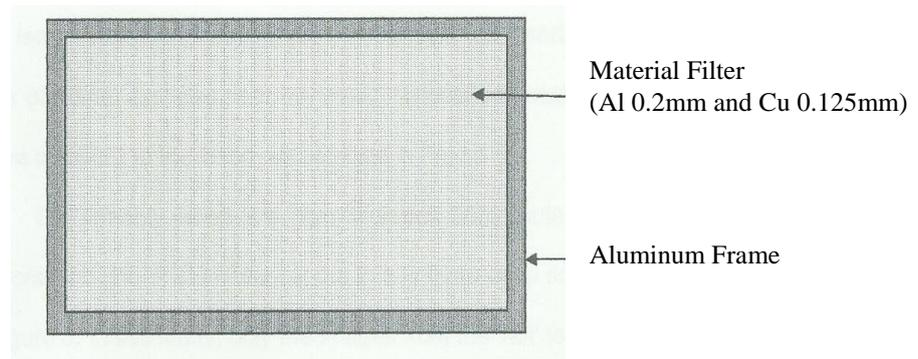
**Fig. 1 Show the design of material filter**
